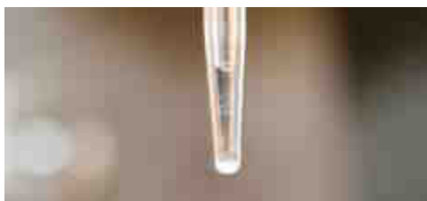
Fig 2.1.13 Last drop of the solution remains in the tip of the pipette
